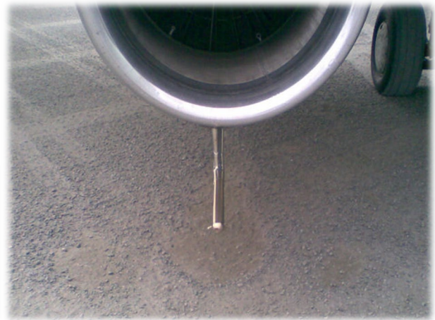
Boeing 737-200 engine anti FOD ingestion protection (tube which blows pressure regulated (55psi) engine bleed air down and aft from 3 nozzles at the tip to break up the vortices)
