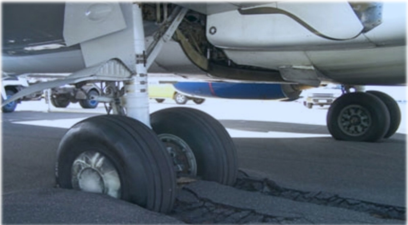
Loose surface material or a failure of surface strength can cause a plane's tires to literally sink into the airstrip, trapping it.
