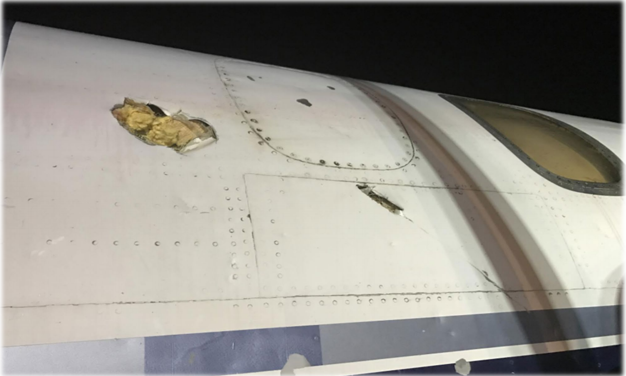
Example of FOD-related heavy aircraft skin damage
